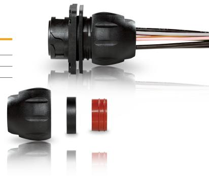
As an accessory for the panel mount connectors of the 696 HEC series Binder offers a sealing kit consisting of a pressing screw, thrust collar and a sealing for the single wires. This set allows effective protection against humidity also at the cable outlet.
